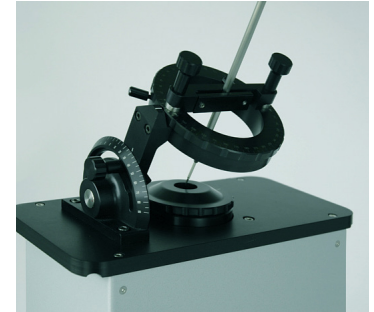
The pitch-yaw manipulator used for directional calibration of multi-wire probes.
