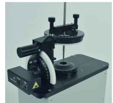
The Automatic Directional Calibrator performs directional calibration of multi-wire probes.
