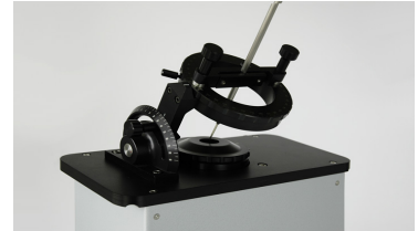
Manual Directional Calibrator mounted on top of an automatic calibrator. It allows probe rotation around two axes.
