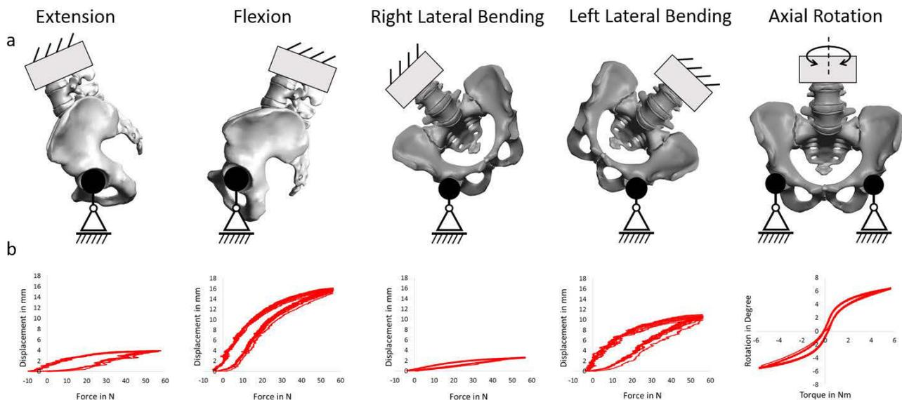
**Figure 2:** Tested loadcases: a – pictograms of loading scenario; b – evaluated cyclic force-displacement diagrams of complete specimen during each loadcase.
