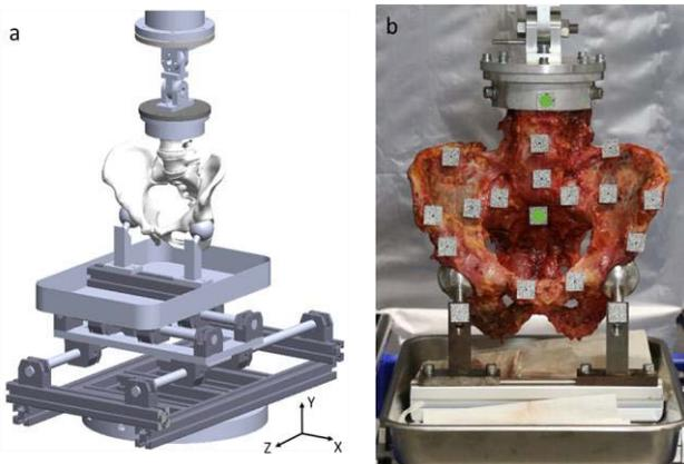
**Figure 1:** Experimental setup: a – CAD-concept of the experimental setup; b – Human bone and soft tissue specimen including measurement markers at anatomical landmarks, evaluated markers of the current study are indicated with a green dot.
