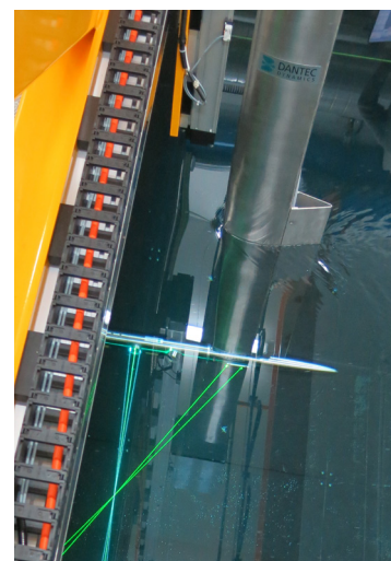
The probe is attached to a streamlined strut (optional) connected to a traverse (optional).
