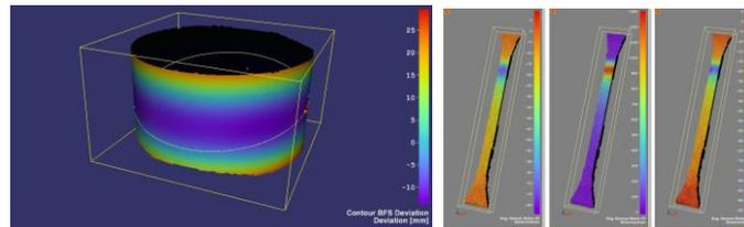
**Fig. 1.** Full-field evaluation of a cylindrical object with an 8 camera DIC System (left image). On the right - tensile test of flat specimen with use of 4 camera system in bi-plane configuration. Strain distribution in X, Y and Z (thickness) direction (right 3 images).
