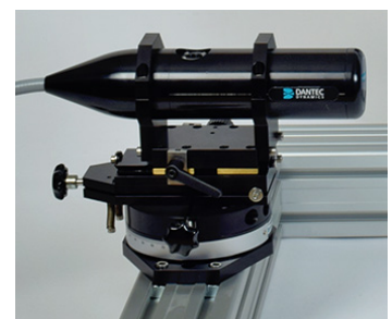
FiberPDA receiver probe with rotation, tilt and translation support for alignment with LDA transmitter.
