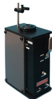
*Hotwire Calibrator for manual velocity calibration.*
