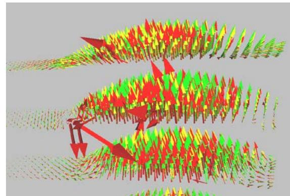
**Fig. 12:** Simulated comparison vector results demonstrate the improvement Volumetric Calibration Refinement. Red: Velocities from outdated initial calibration. Green: Velocities from simulated voxel space. Yellow: Velocities from refined calibration.
