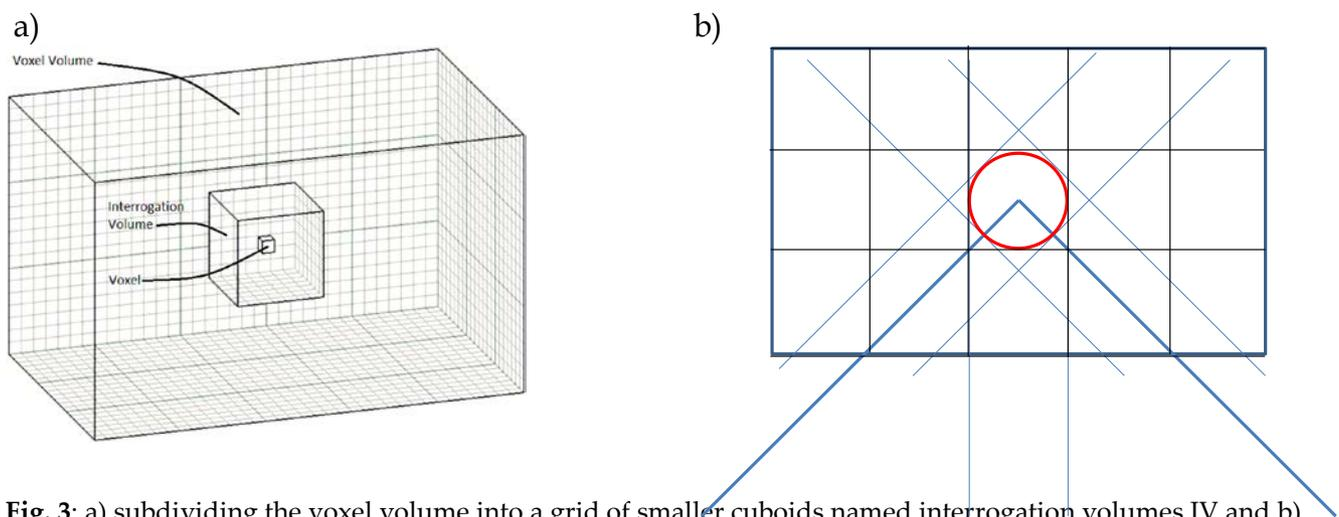
**Fig. 3:** a) subdividing the voxel volume into a grid of smaller cuboids named interrogation volumes IV and b) masking a spherical box around the center of the IVs (red circle in top view) prior to back-projection of the IV into the image planes. This ensures that only those voxels inside the spherical volume of the IVs are contributing to the intensity in the projections.
