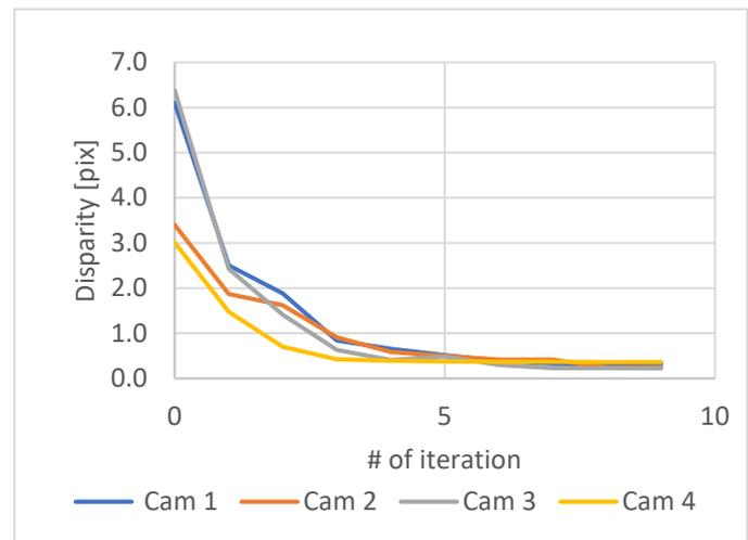
**Fig. 9:** Maximum disparity error over the number of refinement iterations
