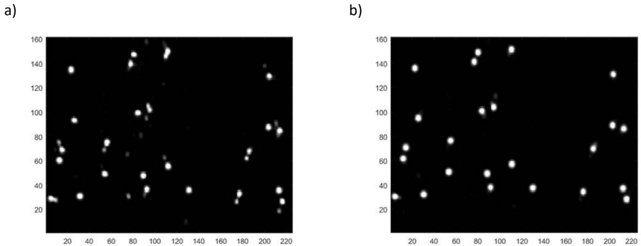
**Fig. 7:** Top view of MART reconstruction of particle field in the three-cam arrangement shown in Fig. 1. a) reconstruction with initial error in calibration with 3px error shift in cam#1, showing larger number of ghosts. b) reconstruction after final iteration step in Fig. 6.
