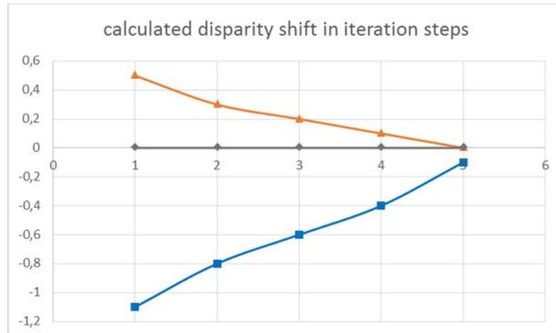
**Fig. 6:** Iterative reduction of residual disparity shifts in all three cameras after inducing an initial 3px mismatch in cam#1 in positive direction along the long axis of the camera, see Fig 1b (blue: cam#1, orange: cam#2, gray: cam#3).
