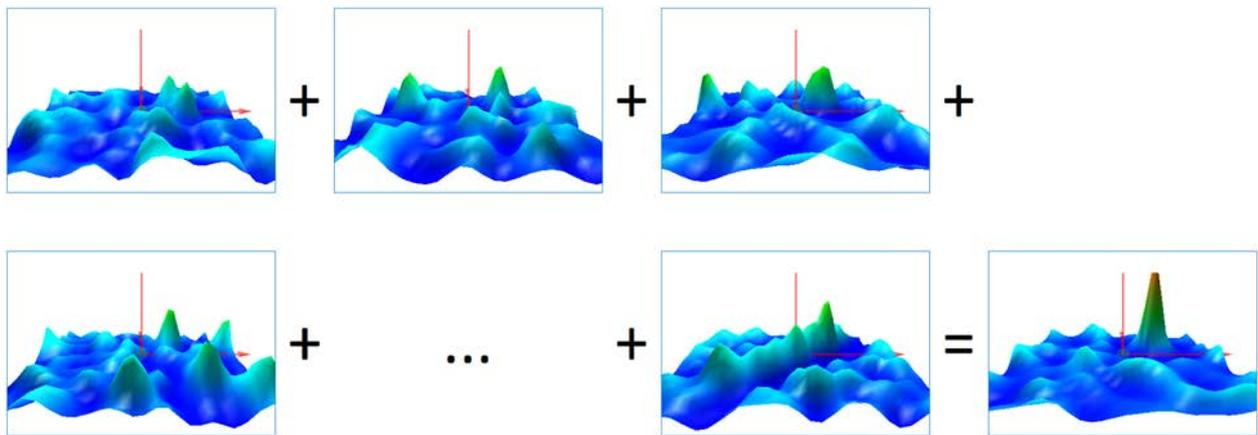
**Fig. 4:** Addition of the correlation maps for the same IV and camera, obtained from different sets of particle images. The resulting peak represents the disparity shift in the image plane for the given center-location of the IV in the reconstructed voxel volume.
