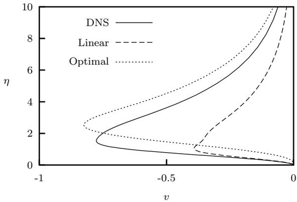
Figure 10: Comparison of wall-normal velocity profiles for  $x = 335$  mm,  $Re_k = 119$ .
