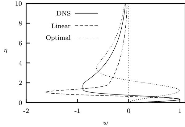
Figure 11: Comparison of spanwise velocity profiles for  $x = 335$  mm,  $Re_k = 119$ .
