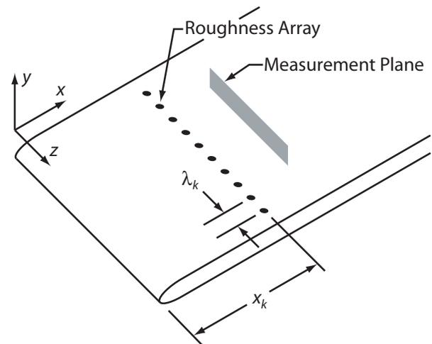
Figure 1: Schematic view of the flat plate model and roughness array.
