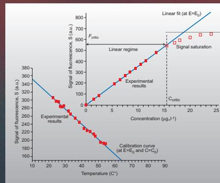
Typical single-pixel temperature and concentration calibration curves
