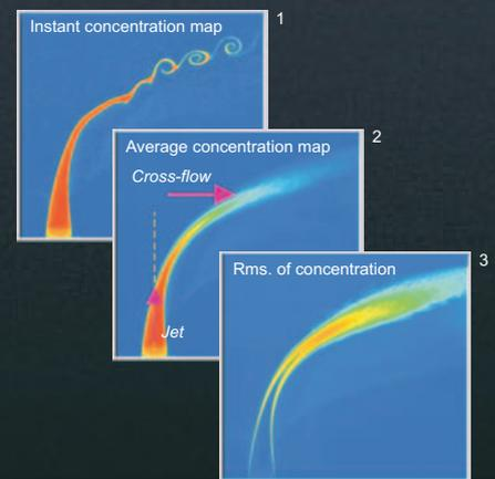
Example of instant and statistical maps of concentration obtained with planar-LIF measurements
