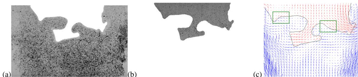
**Figure 2** Application of phase separated PIV measurements in a swirling flame ( $t=5$ ms in Ref. 3). (a) 1<sup>st</sup> frame of the fuel phase of the raw particle image pair, (b) same for the combustion products phase (c) Close up of the phase-separated PIV measurement results at the same instant. Red vectors are in the products phase, blue vectors are in the fuel phase, and the black continuous line is the phase boundary.
