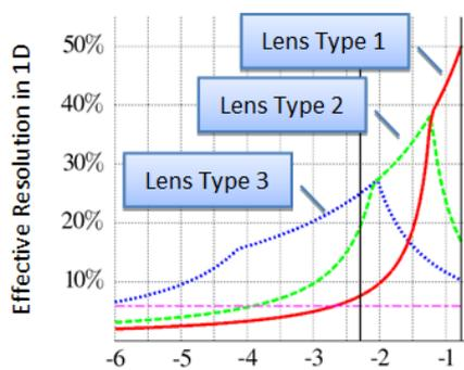
**Figure 2.** Resolution versus depth (courtesy Raytrix)
