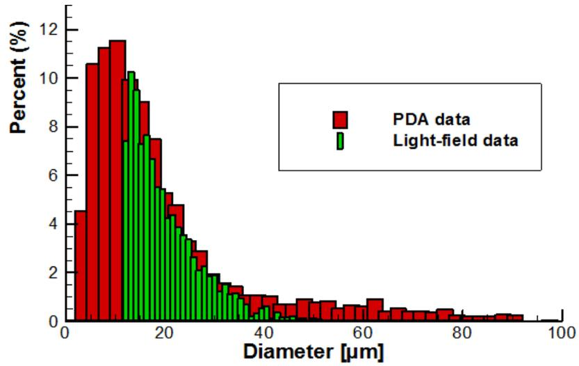
**Figure 10.** Comparison of spray particle diameter distributions between data acquired from PDA and Light-field camera.
