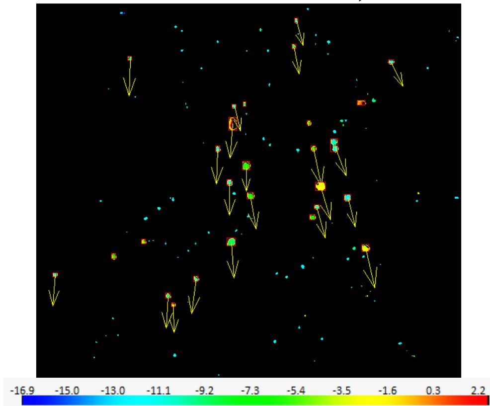
**Figure 9.** Subset ROI of spray with color mapped depth and 2D vectors.
