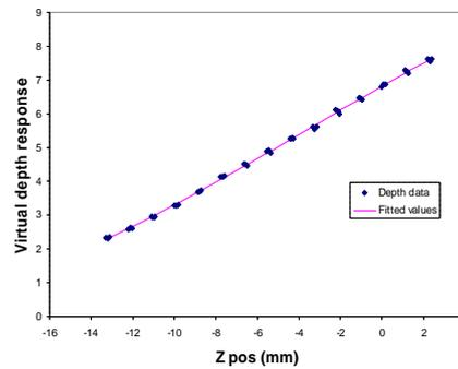
**Figure 6.** Calibration fit between virtual depth and measured depth.
