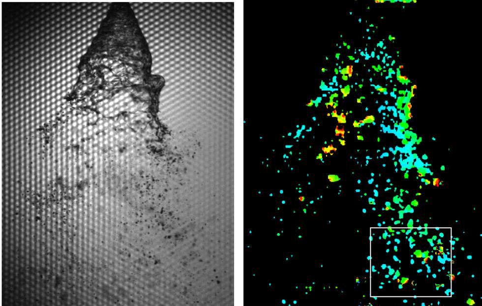
**Figure 8.** Focus and color-mapped depth map of spray from light-field results.
