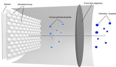
**Figure 1.** Optical schematic of light-field principle.
