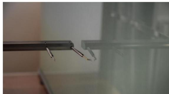
**Fig 2b** Hotwire probes during boundary layer measurements.
