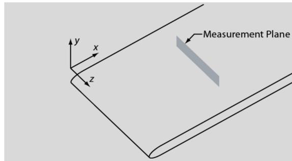
**Fig 2a** The flat plate schematic, the assumed coordinate system and the measurement plane.
