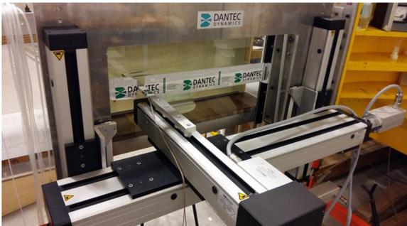
**Fig 1a** Computer controlled, 3-axis traverse system mounted on the DTU wind tunnel.
