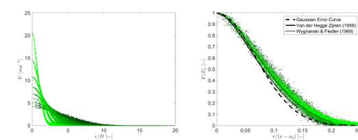
Figure 4 Unscaled (left) and similarity scaled (right) streamwise velocity ( $U$ ) profiles.
