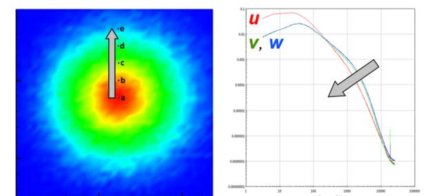
Figure 6 Left: PSD computation positions at  $x=30D$ . Right: Power spectra for  $u$ ,  $v$ , and  $w$  at 30D on the jet centerline. Arrow on the right indicates the movement of PSD results as the measurement point moves from a to e.
