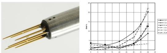
Figure 2 Left: New triple-sensor probe with straight prongs. Right: Error variation with incidence angle.
