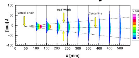
Figure 3 Jet profile development in downstream direction  $x$ . Nozzle located at (0;0)
