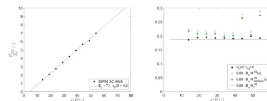
Figure 5 Left: Centerline velocity change in  $x$ . Right: Momentum flux conservation in  $x$ .
