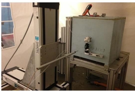
Figure 1 Jet facility, hot-wire probe and 3-axis traversing mechanism.
