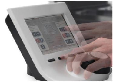
*Control device with display for easy motorized control of microscope*
