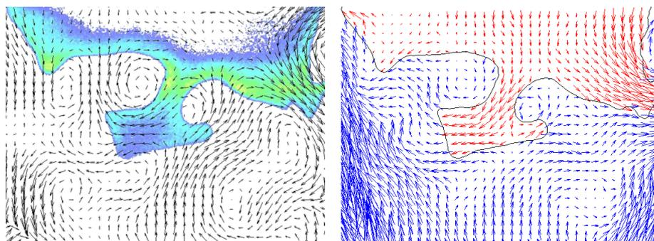
*Left: A single frame from simultaneous TR OH LIF and TR PIV in a lifted flame. Right: Flame front detection using OH LIF (black line), allowing phase separated PIV analysis in the burnt (red) and unburnt (blue) regions, for improved PIV result.*
