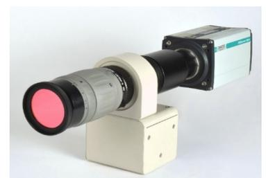
*HiSense Zyla camera, image intensifier unit and front lens*
