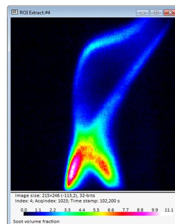
*Soot-volume-fraction measurement in a sooting diffusion flame.*
