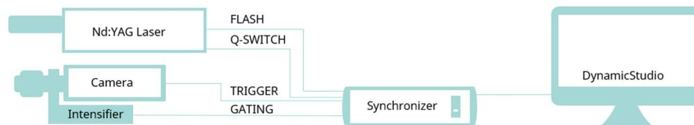
*Overview of the different components, timing and data flow.*
