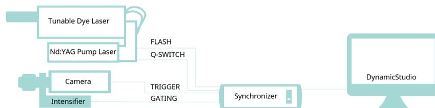
Overview of the different components, timing and data flow.
