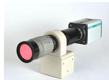
*HiSense Zyla camera, image intensifier and UV front lens*
