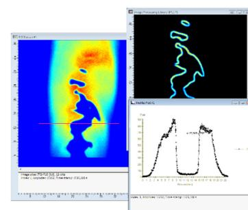
*OH distribution in a Bunsen type flame, including a cross-section intensity plot and the result of gradient detection showing the main reaction zone.*
