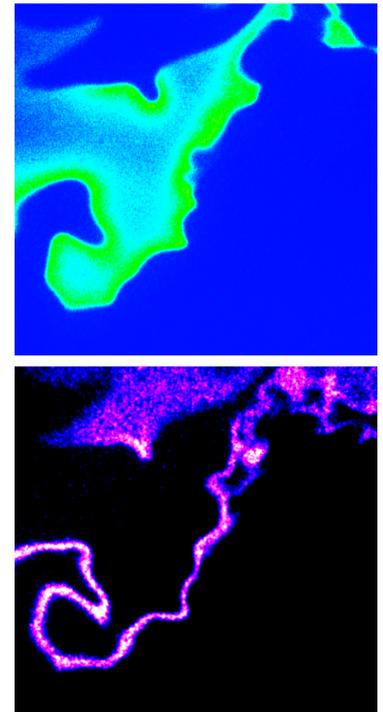
Simultaneous dual-species PLIF by two synchronized systems, showing the flame front and postflame gases (OH, top) and the pre-heat layer (CH<sub>2</sub>O, bottom) in a turbulent lab flame.
