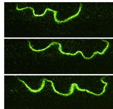
*LIF imaging of CH showing the thin flame front at the base of a turbulent gas flame.*
